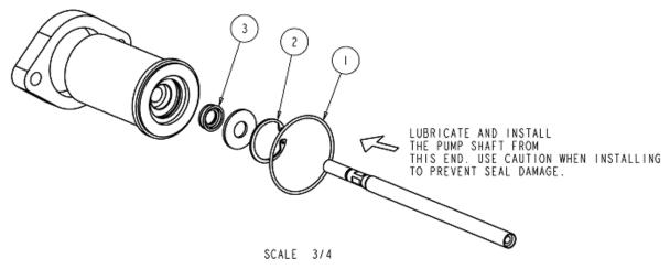
Figure 48: PR70 Rear Pump Rebuild Kit (LC0094)
